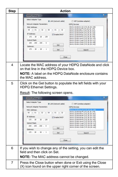
Once the HDPQ DataNode is set up, connect to the instrument to verify the settings.
