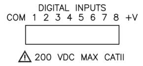
**CAUTION** The +V output terminal is rated +5V, 100 mA Max
