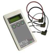
Small, portable, 3-phase true RMS current data logger
