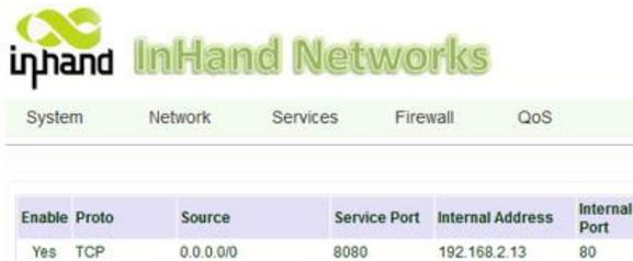
Figure 3. Cellular Router Port Mapping
