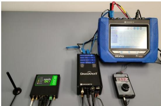
Figure 4. DranXperT & HDPQ Plus Sharing a Cell Router
