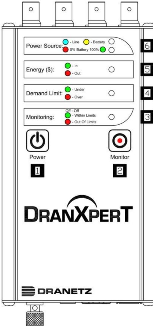
**1 Power Button** – press to turn the instrument power ON or OFF
