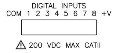
**CAUTION** The +V output terminal is rated +5V, 100 mA Max
