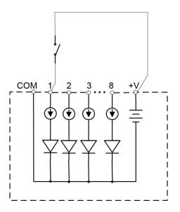
**External Supply** If an external voltage supply is used instead of the +V output, the "COM" terminal must be connected to the external common of the digital power source.
