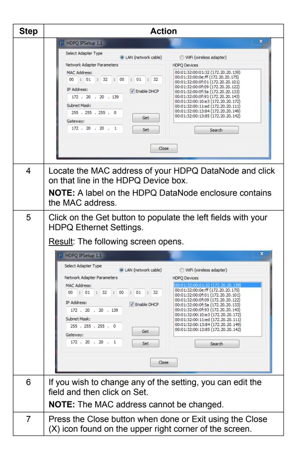
Once the HDPQ DataNode is set up, connect to the instrument to verify the settings.
