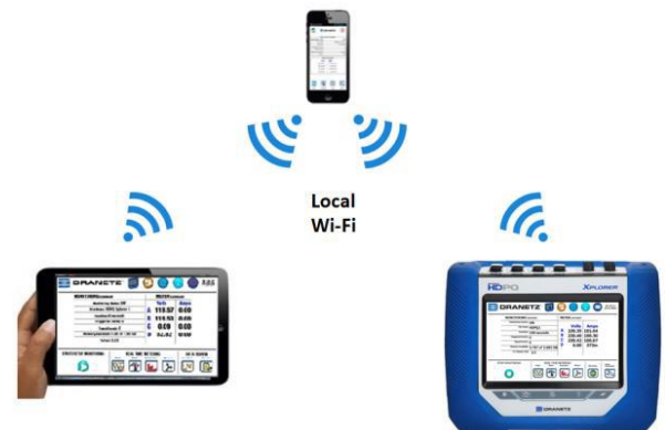
Figure 2. Dranetz HDPQ remote communications with a Tablet & Smartphone.
