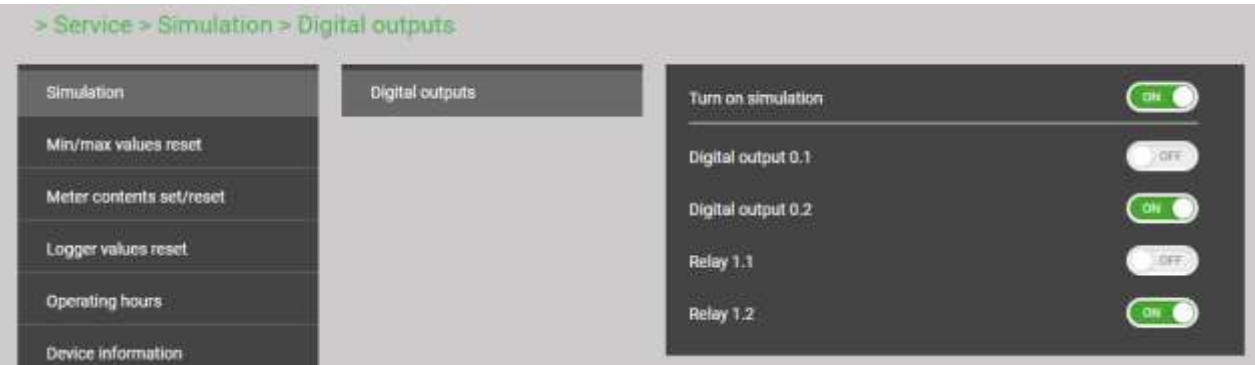
Simulation of digital outputs via device webpage
