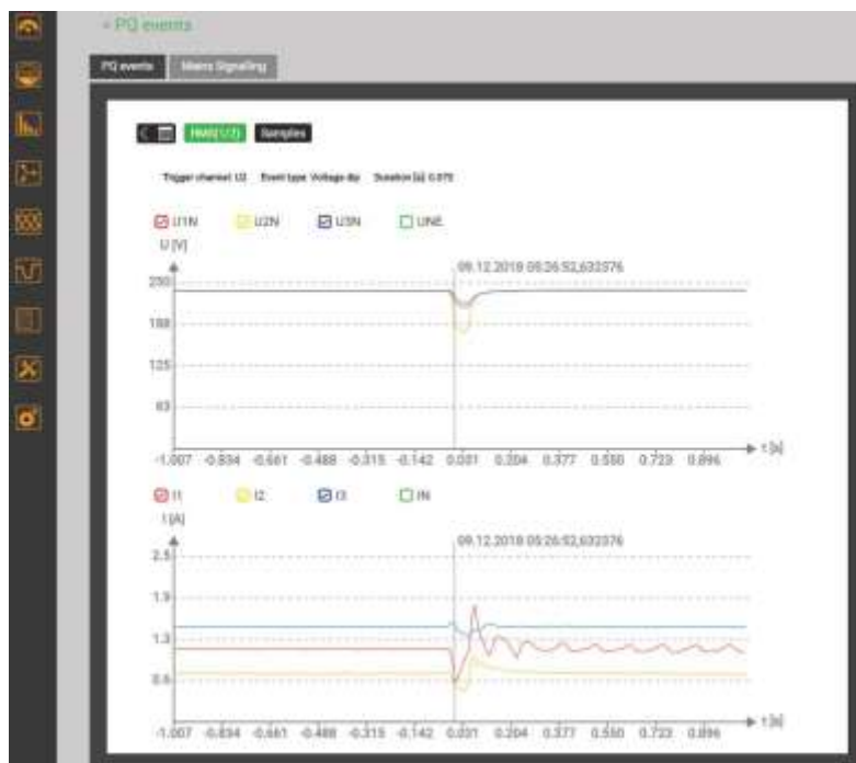
Graphical display of a disturbance recording
