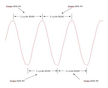
When a trigger occurs, data is stored to memory in accordance with the RMS Summary and Waveform (# of cycles recorded) settings entered during instrument setup. Note that the instruments also detect and record <u>current</u> RMS events in the same manner as voltage. Please see the instrument's users guide for further details.
