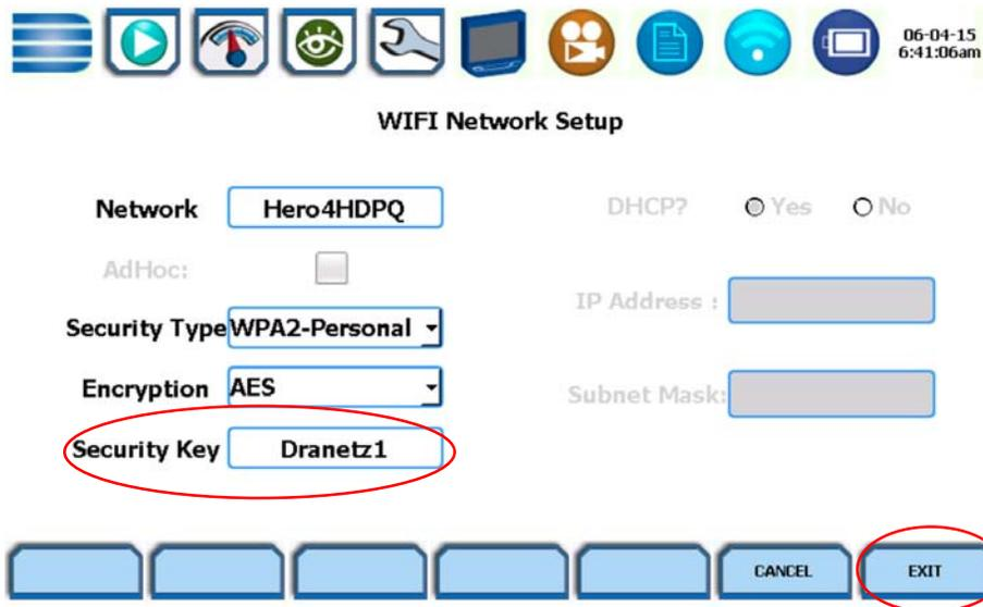
Next press the “Exit” button and the following screen appears and shows that the GoPro camera has connected to the HDPQ instrument.
