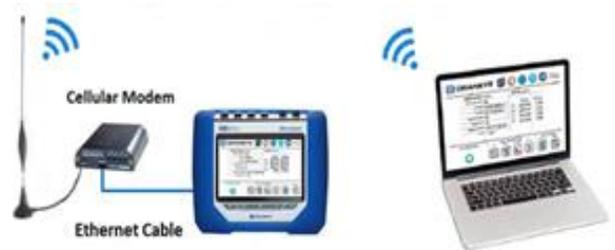
Figure 1. Typical Wireless Modem Application
