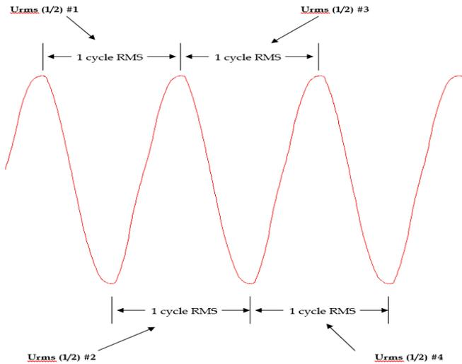
When a trigger occurs, data is stored to memory in accordance with the RMS Summary and Waveform (# of cycles recorded) settings entered during instrument setup. Note that the instruments also detect and record current RMS events in the same manner as voltage. Please see the instrument's users guide for further details.
