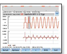
channels to demonstrate that power mitigation devices such as UPS's and stand-by generators are operating properly. Real time readings observed during maintenance and startup processes enable users to see results and tweak that equipment during the testing process.
