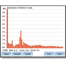
imperceptible variations in performance that can aggregate and cause significant long-term damage. Current harmonics generated by a source can pollute the entire power system. The Power-Visa captures detailed harmonics, interharmonics and subharmonics to effectively troubleshoot the complex problems caused by these events.
