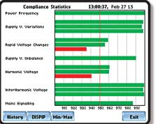
quality. In an instant, the PowerVisa provides a snapshot of over 13 key parameters, including unbalanced voltage variations and harmonics.
