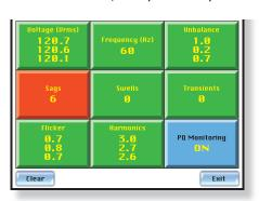
to quickly identify areas of concern, which are identified in red. Drill down for more detailed information by simply touching the intuitive graphical screen to troubleshoot problems, locate the source and pinpoint the root cause of power quality disturbances.
