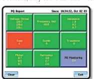
identify areas of concern, which are identified in red. Drill down for more detailed information by simply touching the intuitive graphical screen to troubleshoot problems, locate the source and pinpoint the root cause of power quality disturbances.
