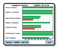
international quality-of-supply standards and benchmark power quality. In an instant, the PowerGuide provides a snapshot of over 13 key parameters, including unbalance, voltage variations and harmonics.
