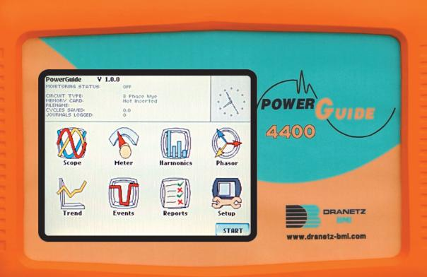
"Out of the Box and Ready To Go," 3-phase, 8-channel **Power Monitoring Instrument**
